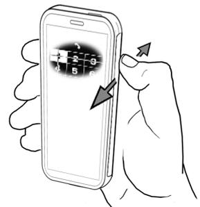
While the user touches the edge-side of the device, a graphical markup (such as the white hair-cross in the figure) is shown on the screen corresponding to the currently touched position. Once the touch is released the highlighted user interface element is selected. Thus the user can correct any wrong selections before releasing the touch.
